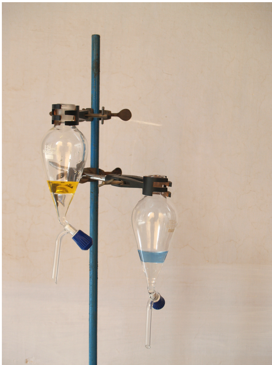
Plate 3.3 Photograph of experimental setup for the separation of organic and aqueous phases
