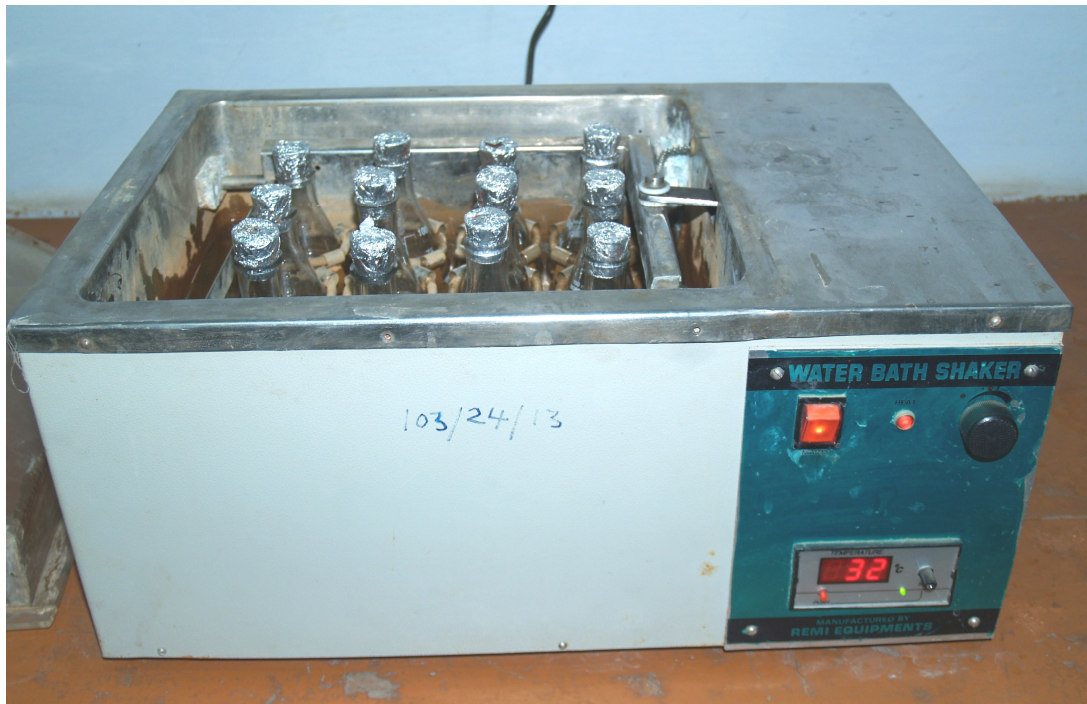
Plate 3.2 Photograph of equilibrium experimental setup with controlled temperature
