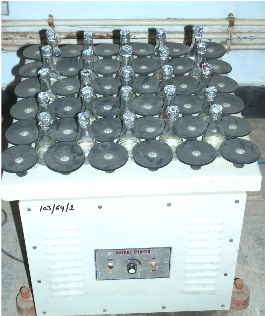
Plate 3.1 Photograph of equilibrium experimental setup at room temperature
