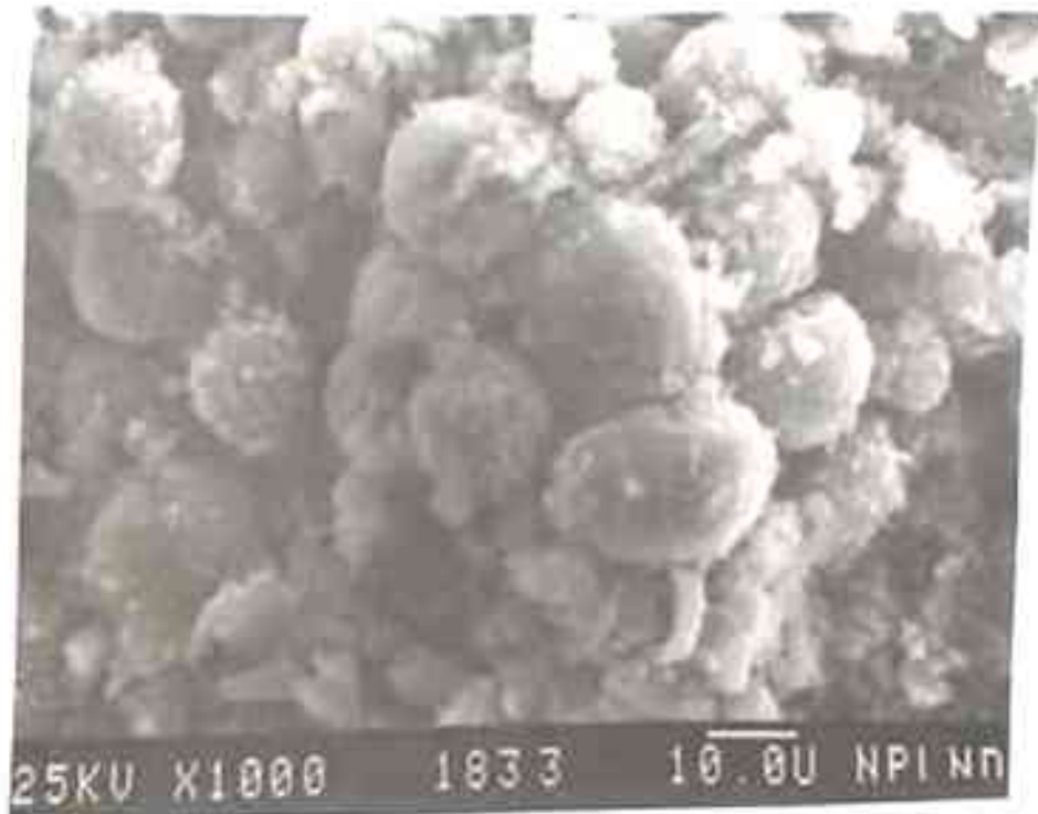
Fig 4.3 Scanning electron micrograph of mesocarbon microbeads separated from the heat-treated pitch.
