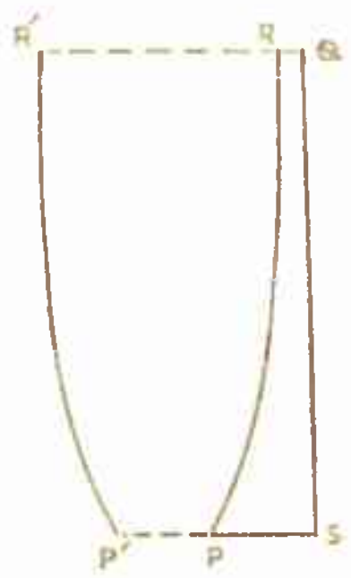
FIG. 2.3 TRANSVERSE CROSS-SECTION OF THE CONCENTRATOR SHOWING THE SHAPE OF THE RIB ON RIGHT SIDE
