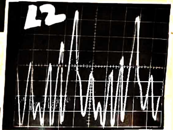
Fig. 6.10 Torque Pulsations 30.0% at 45Hz, 3.0 ft.lb load torque X = 4.5 x 5 msec., Y = 7.2 x 0.1
