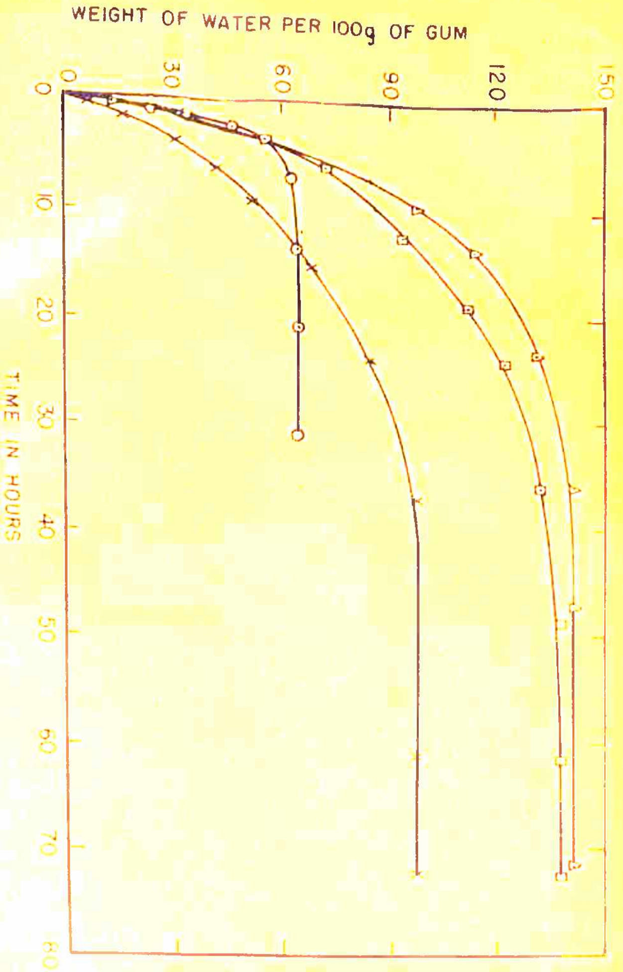
FIG. 5. TIME - SORPTION CURVE OF WATER AT SATURATION PRESSURE ON ACACIA X, PROSOPIS SPICIGERA Δ, GHATTI ◉ AND TRAGACANTH GUM ◻.
