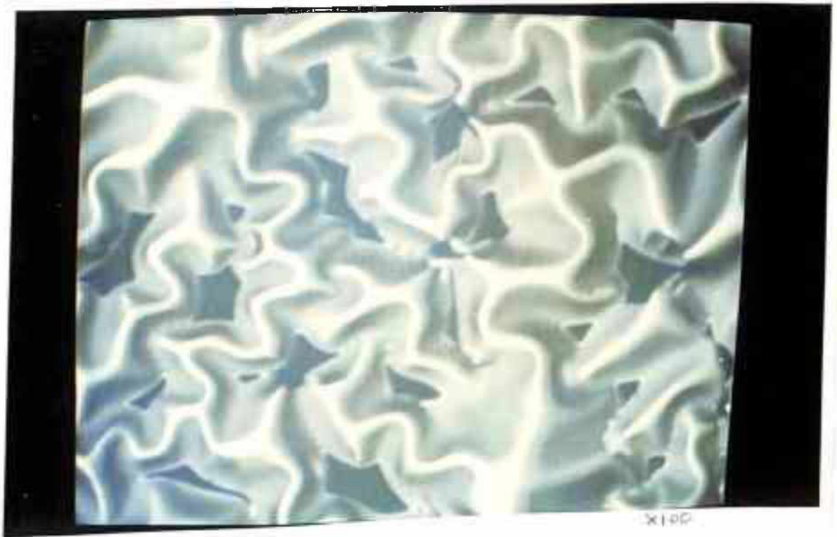
Plate 4.2 Total delamination of DLC film
