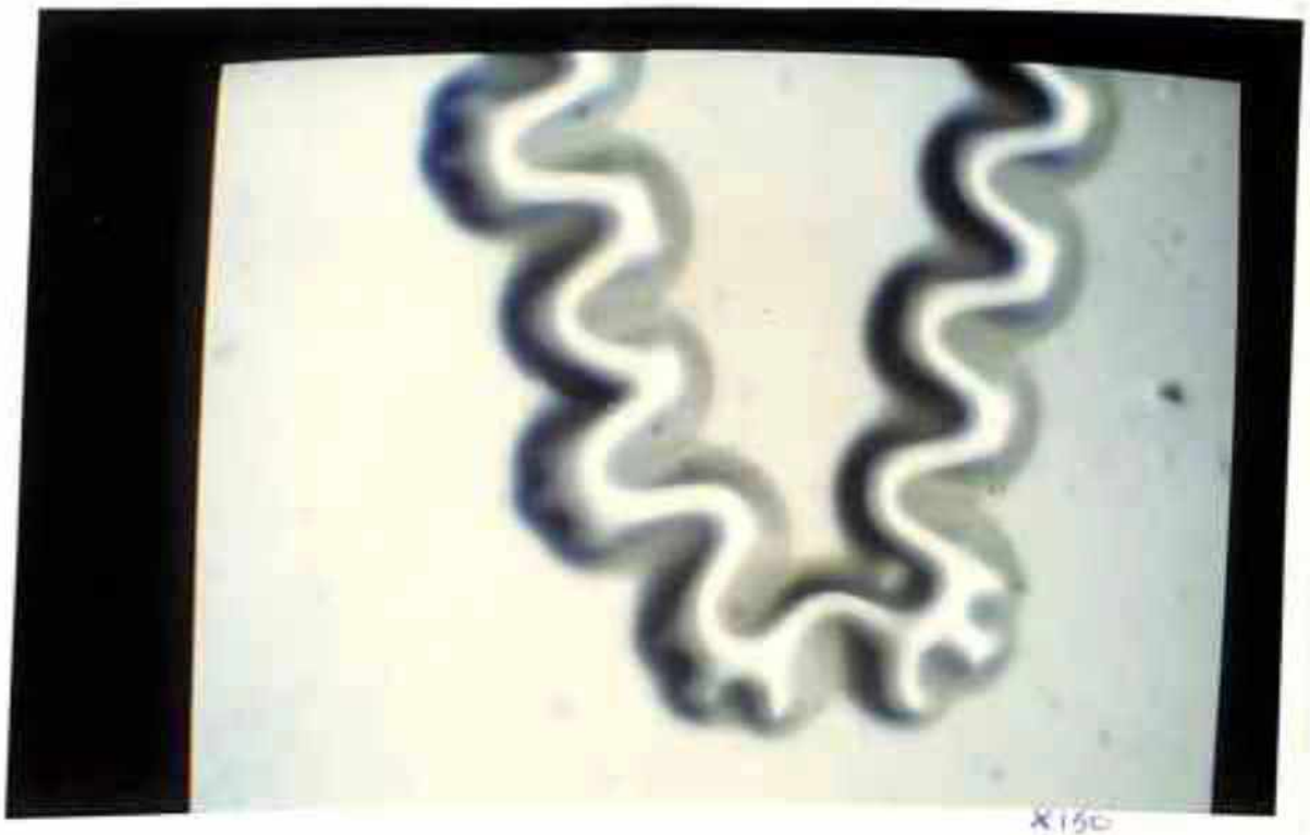
Plate 4.1 Sinusoidal buckling wave stress relief pattern of DLC film
