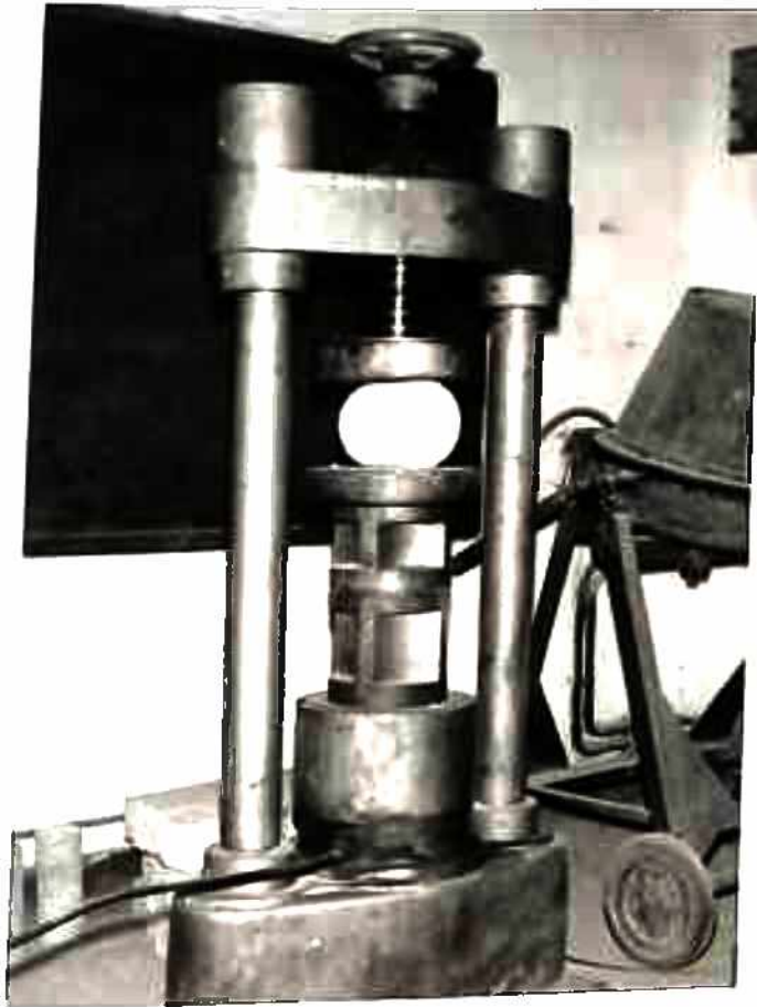
PLATE 3.4 PLAIN CONCRETE CYLINDER UNDER TEST FOR SPLIT TENSILE STRENGTH.
