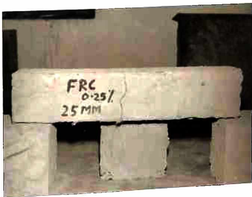
PLATE 7.4 CRACK PATTERN OF SAN FIBRE REINFORCED CONCRETE BEAM ( FIBRE 0.25% ) AFTER FLEXURAL TENSION.
