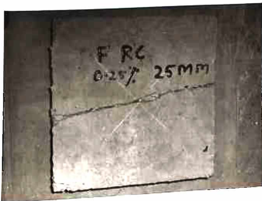
PLATE 8.2 CRACK PATTERN OF SAN FIBRE REINFORCED CONCRETE SHEET ( FIBRE 0.25% ) AFTER IMPACT FAILURE.
