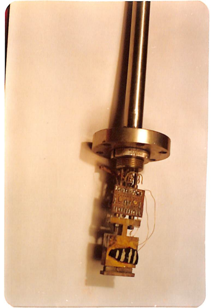
Fig. 3.10. The laboratory designed cryostat used for R vs. T measurement. The photograph at right shows the close view of a typical four probe sample connection on the cryostat.
