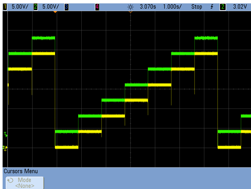
FIGURE 6.9: Measured results voltage across balance switches during balancing
