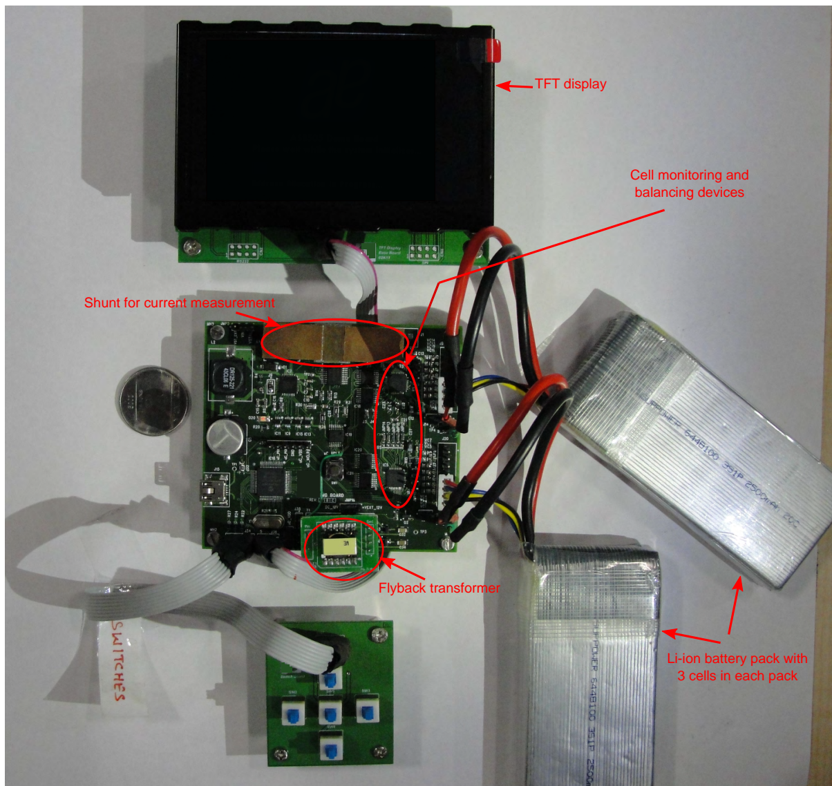
FIGURE 6.2: Demo board setup with 3 cells in each pack
