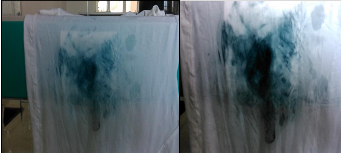
Fig.6.6: Cloth dyed by direct spraying of bio- indigo with silicon oil
