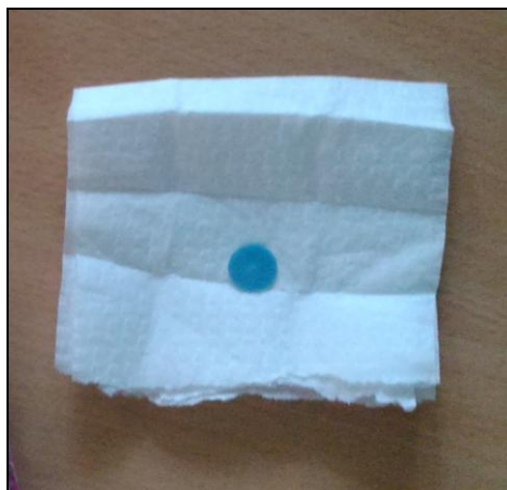
Fig.5.4: Pellet of blue pigment Indigo along with KBr
