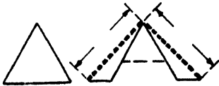
(c) Three-phase to two-phase, with the small phase-winding divided into two equal parts and connected as shown. Same as one-half of fig. 50 (2).
