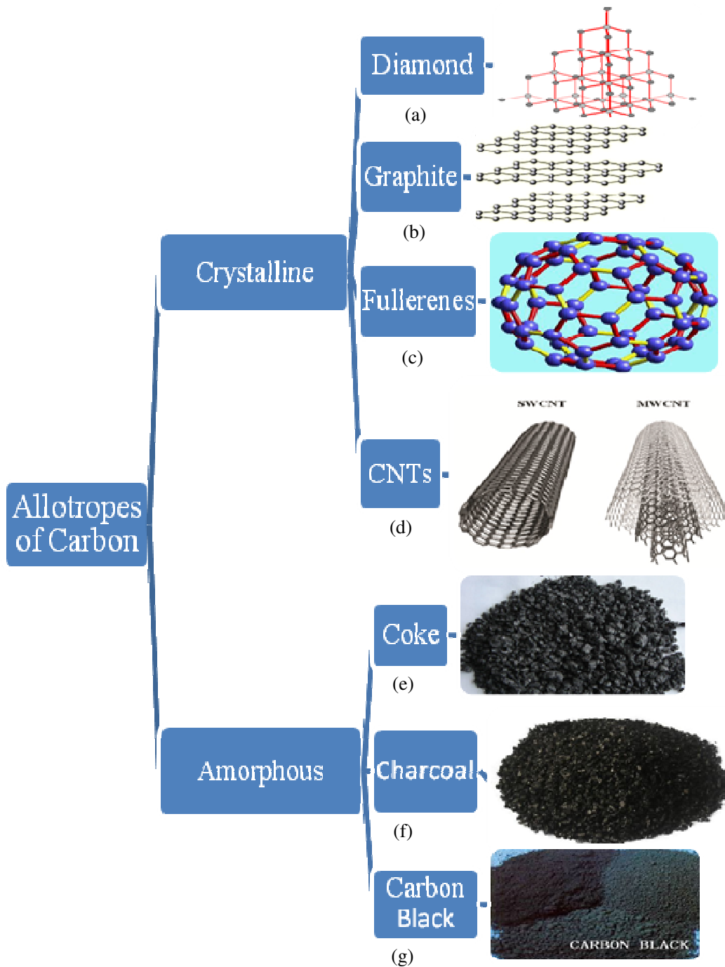
Figure 1.1: Allotropes of carbon (a) Diamond [1] (b) Graphite [2] (c) Fullerenes [3] (d) CNTs [4] (e) Coke [5] (f) Charcoal [6] (g) Carbon Black [7]
