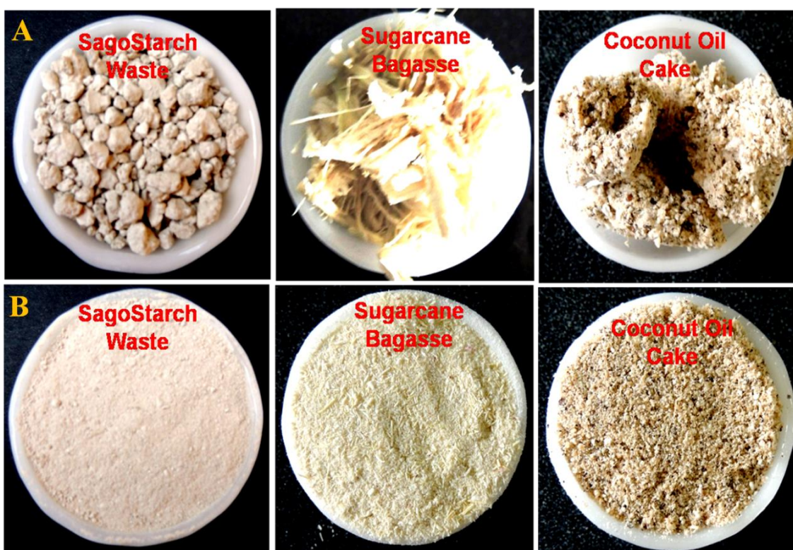
Fig. 6.1 Agro-industrial wastes, SSW, SCB, COC (A) procured form and (B) pulverized form.
