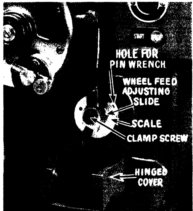
FIG. 379. MECHANISM FOR ADJUSTING AUTOMATIC CROSS FEED
