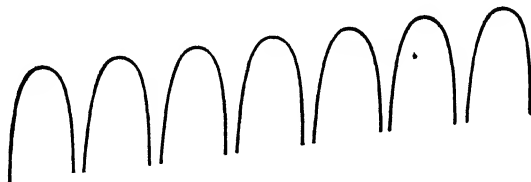
Fig. XXIX-2.—Potential energy of an electron in a field representing a metal with a current flowing, and an average potential gradient.
