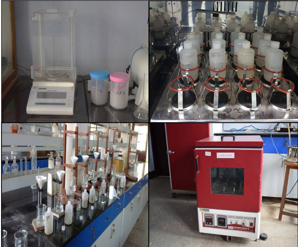
Fig. 4.3 Batch leaching test performed in the laboratory
