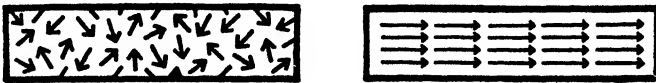
FIG. 23.—The theory of magnetism—a steel bar (left) becomes magnetized (right), and the tiny particles all point in one direction.
