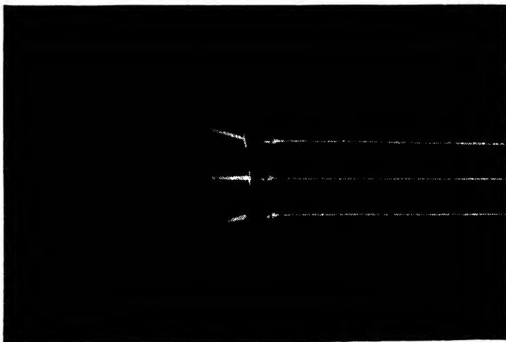
FIG. 61.—Refraction of parallel light beams through a concave or diverging lens. (Courtesy of the Museum Committee, Massachusetts Institute of Technology.)
