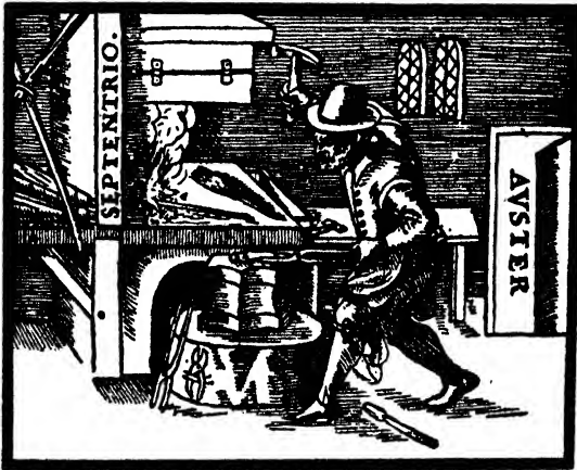
FIG. 261. Effect of hammering and heating on magnetization.
