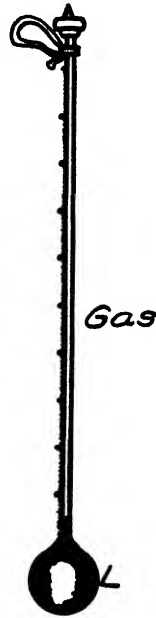
FIG. 217. The first sealed thermometer (1665).
