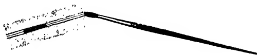
Fig. 34. Location of colorless adsorbed compounds by brushing on a reagent that forms a colored product (Zechmeister, Chohnoky and Ujhelyi).
