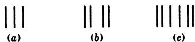
FIG. 111. ZEEMAN PATTERNS. (a) "Normal" Zeeman pattern. For the Hg singlet line at 5790Å, and H = 10,000 oersteds, the lines are separated by 0.156Å. (b), (c) Two examples of "abnormal" patterns.
