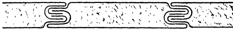
Fig. 38. One form of connection of negative pockets in plates of nickel-cadmium batteries.
