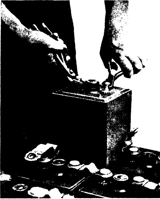
FIG. 97. Removal of cell from the battery. If the jar sticks, a hot putty knife may be inserted around the edges.
