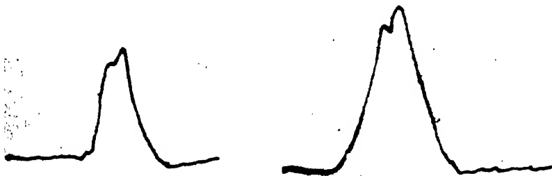
Fig. 5.6—Oscilloscope records of two x-ray pulses from a tube operated by a 370-kv Westinghouse impulse generator. Total duration of the sweeps 4.4 \mu\text{sec} . X-ray tube 21 ft from the ionization chamber.
