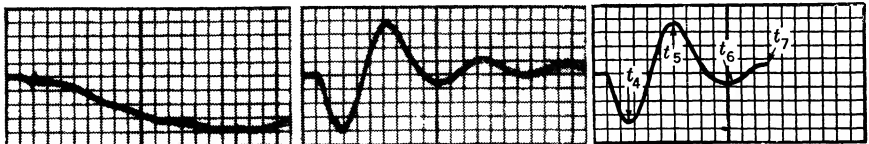
(g) 1\mu sec = 10 div. (h) 1\mu sec = 1 div. (i) Calculated from circuit (f). Current in the 20-mh inductance recharging path.
