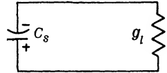
FIG. 2-9.—Equivalent circuit for calculating the trailing edge of the pulse for a hard-tube pulser with a resistance load.
