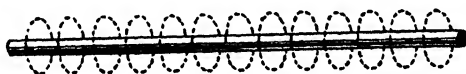
FIG. 12.—A conductor carrying current is surrounded by a magnetic field, which forms a kind of invisible sleeve round it.
