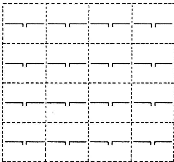
Fig. 3.1. Broadside array. Each dotted square = \frac{1}{2}\lambda \times \frac{1}{2}\lambda (area \frac{1}{4}\lambda^2 ) contains one \frac{1}{2}\lambda aerial. The whole aerial is 2\lambda \times 2\lambda = 4\lambda^2 , n = 16 .
