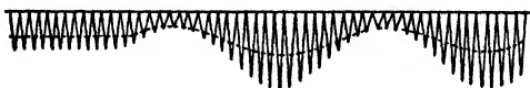
CONTINUOUS WAVES MODULATED AND RECTIFIED DOTTED LINE SHOWS AVERAGE CURRENT THROUGH TELEPHONE RECEIVER
