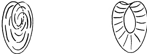
Figure 4.2. Minimal surface forming a Moebius strip and simply connected minimal surface through same contour.
