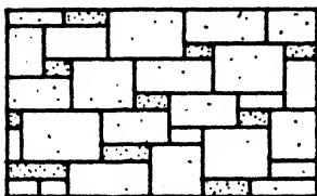
"THREE UNIT"-is stones of three heights have been used.
