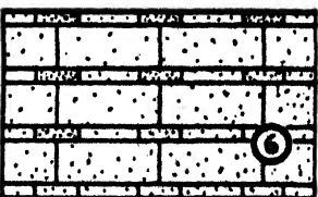
Two heights of stone alternating in a regular arrangement. ALTERNATING COURSED ASHLAR
