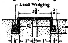
SECTION OF RAGLET (with flashing in place.)
