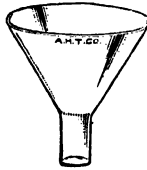
Funnel for transferring powders.
