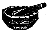
FIG. 128.—Agate mortar for triturating very small quantities of material, particularly samples for quantitative analysis.
