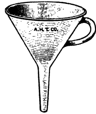
Metal funnel for transferring liquids.
