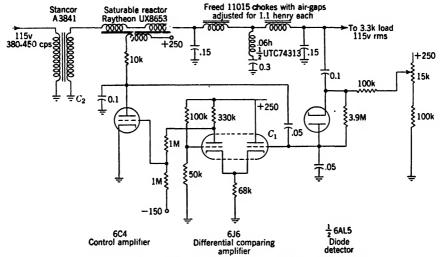
Fig. 16.20.—Degenerative a-c regulator using magnetic saturation.
