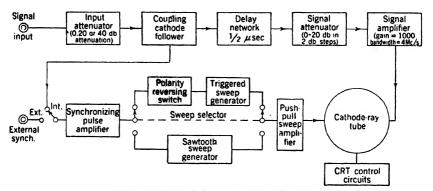
Fig. 18-21.—Block diagram of the TS34/AP.
