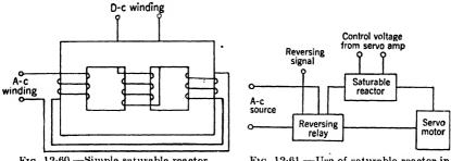
Fig. 12.60.—Simple saturable reactor.
