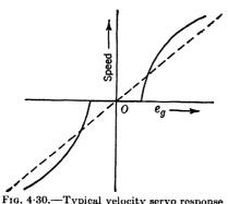
Fig. 4.30.—Typical velocity servo response to error signal.
