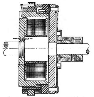
Fig. 12-23.—Moving-coil friction-type magnetic clutch.
