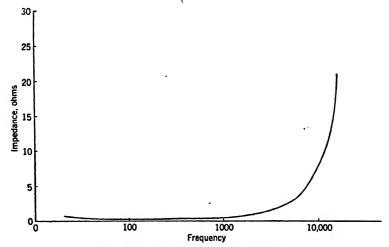
Fig. 16.50.—Characteristics of regulator E.
