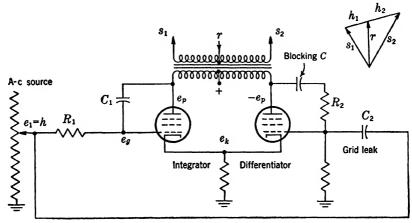
Fig. 6.18.— Phase-shift triangle solver.
