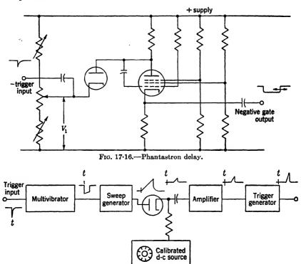
Fig. 17-17.—Linear-sweep delay block diagram.
