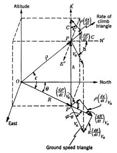
Fig. 7.12.—Simplified system geometry.
