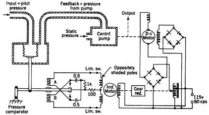
Fig. 14-14.—Ship's log using rate servo.
