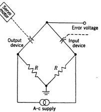
Fig. 12-5.—Use of condensers as data input and output devices.
