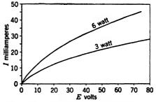
Fig. 15.8.—Volt-ampere characteristic of 110-volt Mazda lamps.
