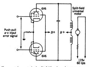
Fig. 12-59.—Vacuum-tube control of split-field universal-type motor operated on a-c. used to control the large amounts of power necessary to operate motors. Relay control of a-c motors is discussed in Sec. 12-24. Saturable transformers followed by contact rectifiers are sometimes used for the control of d-c motors.
