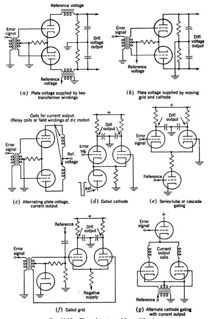
Fig. 12-15.—Phase detectors with amplification.
