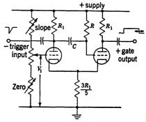
Fig. 17-15.—Delay multivibrator.
