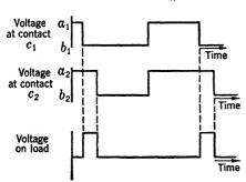
Fig. 12·47.—Voltage waveforms at relay contacts in control circuit for bidirectional control of d-c motors.
