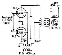
Fig. 12.56 — Airborne servo power stage for 400-cps operation of induction motor.
