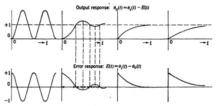
Roots conjugate imaginary Roots conjugate complex Roots real and equal Roots real and unequal Fig. 9.5.—Types of response curves corresponding to different solutions of a second-degree characteristic equation.
