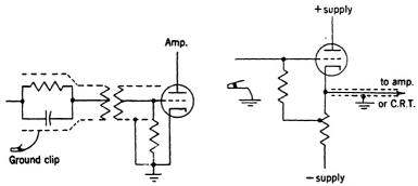
Fig. 17-10.—Voltage-divider probe.
