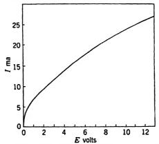
Fig. 15·10.—Volt-ampere characteristics of Victoreen filament-type reference tube. matically in a majority of the circuits. Volt-ampere characteristics for these two Mazda lamps are shown in Fig. 15·8.
