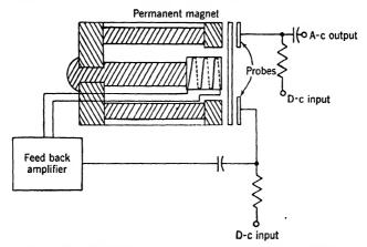
Fig. 15-25.—Modulation circuit employing vibration multiplier.
