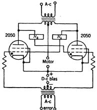
Fig. 12-34.—Unidirectional full-wave thyratron control of d-c motor, using a-c error signal.
