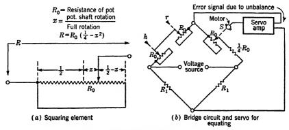
Fig. 6.7.—Triangle solver using resistance squaring and bridge.
