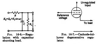
of  $\mu$  and  $g_m$  it is apparent that the per cent regulation is  $1/\mu \times 100$  and the internal impedance is  $1/g_m$ . If a pentode is used, the regulation is
