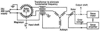
Fig. 12.2.—Use of Magnesyn in servo loop.
