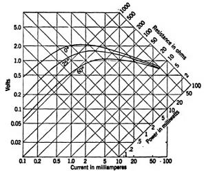
Fig. 15-14.—Variations in Thermistor characteristics with ambient temperature. These data are for D-163903 and D-166382 units.
