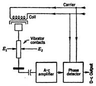
Fig. 15-22.—Switch-type modulator comparison circuit.
