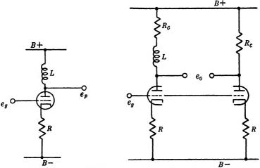
Fig. 4-14.—Cathode-follower RL-differ- Fig. 4-15.—Compensation of coil resistance.
