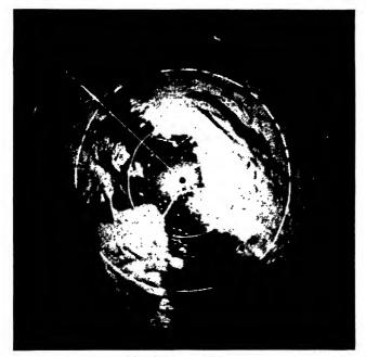
Fig. 7.2.—Radar plan-position indicator with range and azimuth markers.
