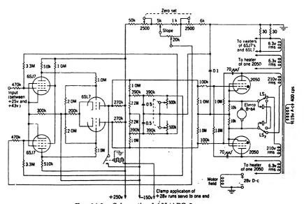
Fig. 14.2.—Schematic of AN/APG-5 servo.
