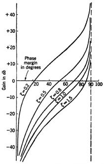
Fig. 10·18.—Phase-margin diagrams for a proportional servo system. Different curves differ in value of the damping ratio ζ. As ζ decreases, the phase margin decreases for a given gain.
