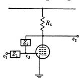
Fig. 6-15.—Single-stage feedback integrator.
