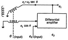
Fig. 5-29.—Device for producing secant and cosecant.
