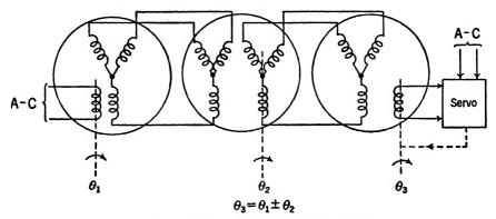
Fig. 3.5.—Addition or subtraction with synchros.
