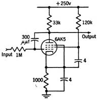
Fig. 6.16.—Integrator circuit.
