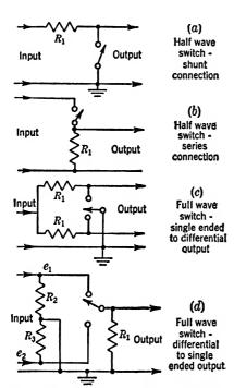
Fig. 12.9.—Typical switch modulator circuits.
