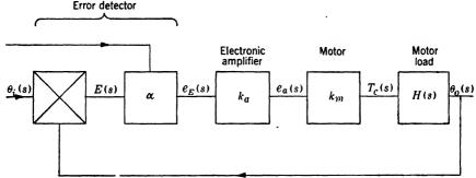
Fig. 11·10. Block diagram of a servo, system with variable loop gain. Symbols:  $\alpha$  is error detector conversion factor  $e_E(s)/E(s)$  in a-c volts per radian error,  $k_a$  is gain of electronic amplifier  $e_a/e_E$  in numerical units,  $k_m$  is motor conversion factor  $T_c(s)/e_a(s)$  in torque units per volt applied, and H(s) is transfer function of output member, in this case the motor load.
