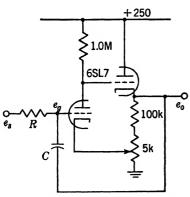
Fig. 4:24.—Integrator with resistive regeneration and cathode-follower output.
