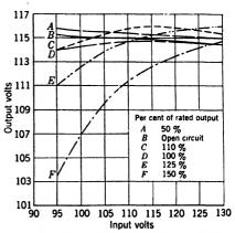
Fig. 16·14.—Typical regulation curves for various unity power factor loads for a standard 500-volt-ampere voltage stabilizer.
