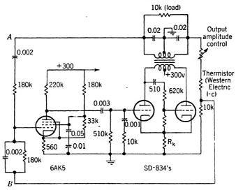
Fig. 7.4.—Oscillator circuit.
