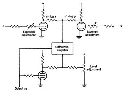
Fig. 5.37.—Use of logarithmic diode characteristics for multiplication.
