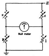
Fig. 1.1.—Simple bridge computer for z = x/y.
