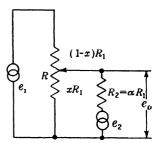
Fig. 5.2.—General loadedpotentiometer circuit with zero-impedance supply.
