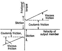
Fig. 11-11.—Diagrammatic representation of types of friction torque.
