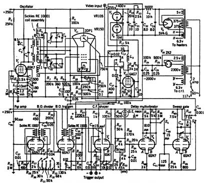
Fig. 18-37.-Model III range calibrator circuit.
