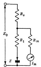
Fig. 5-32.—Voltage divider.  $R_1 = 0$  hmic component of rectifier resistance; Z = logarithmic contact resistance; R = source resistance;  $R_m = meter$  resistance.
