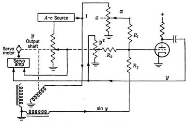
Fig. 6.4.—Circuit diagram of computer for  $y^2 + \sin y + x = 0$ .
