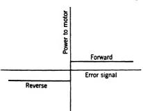
Fig. 12-43.—Relay on-off control characteristics.
