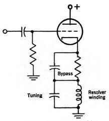
Fig. 5.16.—Cathode-circuit driver.
