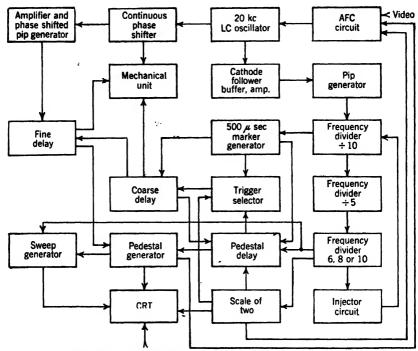
Fig. 19-20.—Block diagram of airborne navigational range unit.
