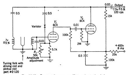
Fig. 16.25.—Constant-frequency oscillator using tuning fork.
