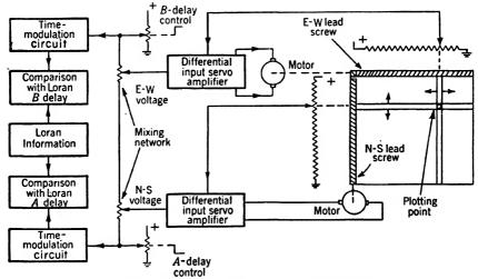
Fig. 6-31.—Schematic diagram of Loran plotting board.
