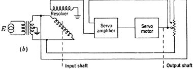
Fig. 12.6.—Examples of variable-gain type nonlinear servo loops.
