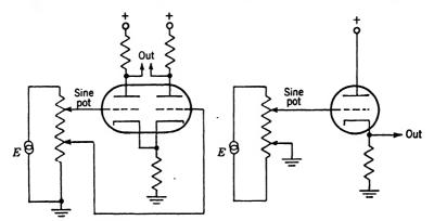
Fig. 5.20.—Sine potentiometer with Fig. 5.21.—Sine potentiometer with floating grounded supply.
