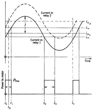
Fig. 12-48.—Graphical analysis of proportional control characteristics.
