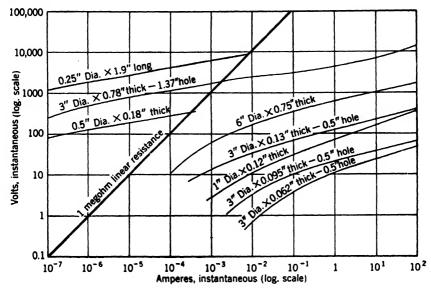
Fig. 15·12.—Volt-ampere characteristics of Thyrite.
