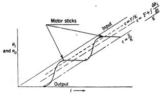
Fig. 11-12.--Servo operation showing effect of stiction.
