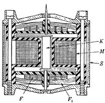
Fig. 12.4.—Cross section of Telegon. (Courtesy of Kollsman Instrument Co.)
