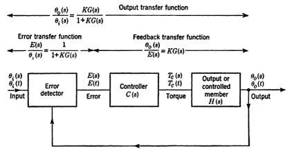
Fig. 9-3.--Block diagram of servo system.
