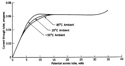
Fig. 15.7.—Volt-ampere characteristics of Amperite ballast tube.
