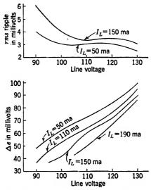
Fig. 16-49.—Characteristics of regulator with balanced comparison circuit.
