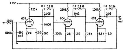
Fig. 7.7.—Step-up driver circuit.
