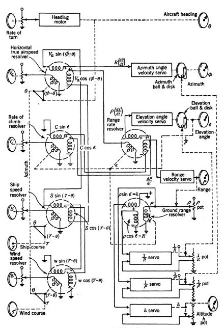
Fig. 7-13.—Simplified block diagram.
