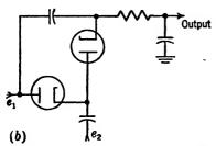
Fig. 6·17.—Methods of combining two voltages differing by 90° in phase. (a) Peak rectifier; (b) double rectifier.
