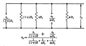
Fig. 5-4.—Transformation of loaded-potentiometer circuit with current generators. ances are all in parallel, the output  $e_o$  is simply the product of the total current and the effective parallel resistance, or
