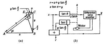
Fig. 6.27.—Loaded-potentiometer triangle solver.
