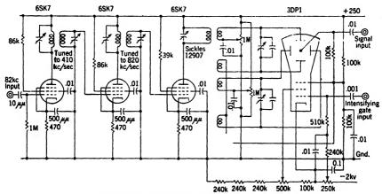
Fig. 18.39.—Circuit of the 200-yd "J" scope.
