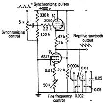
Fig. 17·1.—Free-running thyratron sweep generator.
