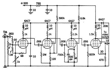
Fig. 18.7.—High-gain video amplifier circuit.
