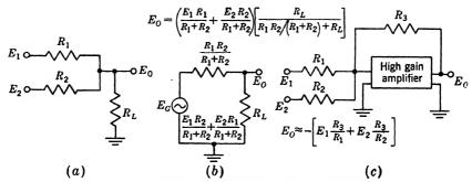
Fig. 3-1.—Addition with parallel impedance networks.
