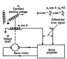
Fig. 5.27.—Device for producing inverse sine and cosine.
