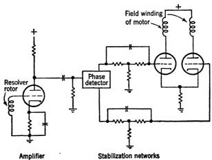
Fig. 7.6.—Resolver servo circuit.
