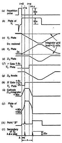
F10. 6·13.—Timing diagram for parabolicsweep triangle solver.
