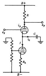
Fig. 4·10.—Cathode-follower differentiator with constant-current tube.
