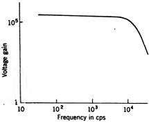
Fig. 18-47.—Gain-frequency characteristic of amplifier without feedback.
