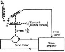
Fig. 5.28.—Device for producing inverse tangent and cotangent.
