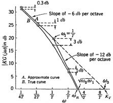
Fig. 10·3.—Gain in decibels vs. log frequency plot of  $KG(j\omega)$ . This may be taken as a plot of  $G(j\omega)$  if the gain constant k or  $k_v$  is unity (0 db), in which case  $\omega_0=1$  radian per second.
