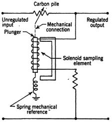
Fig. 15.30.—Carbon pile voltage regulator.
