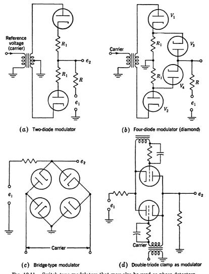
Fig. 12-11.—Switch-type modulators that may also be used as phase detectors. impedances (copper oxide, selenium, or germanium rectifiers, for example) may be used. In the fourth the two triodes together constitute the electronic equivalent of a switch.
