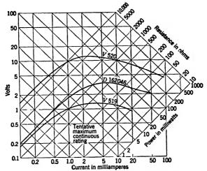
Fig. 15.13.—Typical Thermistor characteristics at 25°C in still air.
