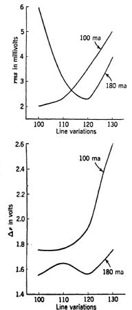
Fig. 16-45.—Characteristics of regulator C.
