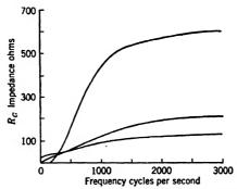
Fig. 16.5.—Internal impedance of VR-105's vs. frequency.
