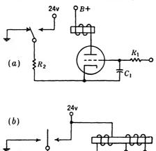
Fig. 12.51.—AN/APA-46 antenna-control servo using two mercury contact relays.
