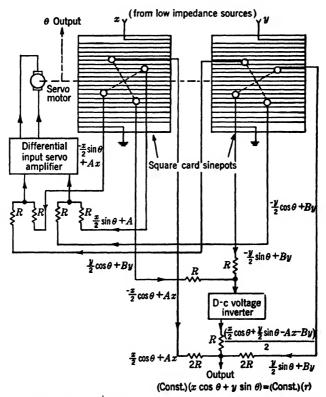
Fig. 6.26.—Rectangular-to-polar transformation using direct voltage.
