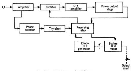
Fig. 7.18.—Velocity servo block diagram.
