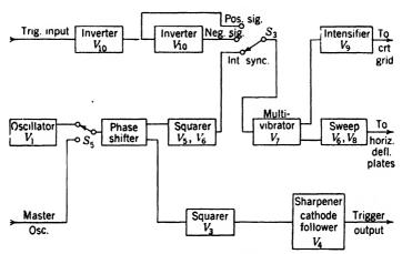
Fig. 18-2.—Block diagram of the P4 synchroscope.
