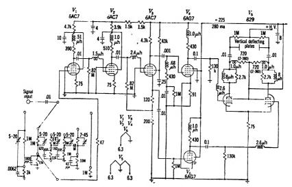
Fig. 18-14.-Wide-band video amplifier circuit.
