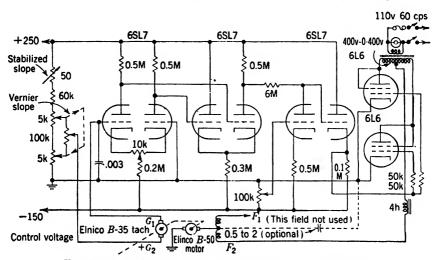
Fig. 12:36.—Full-wave unidirectional velocity servo using 6L6's.
