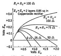
Fig. 5.34.—Characteristics of bridge circuit.
