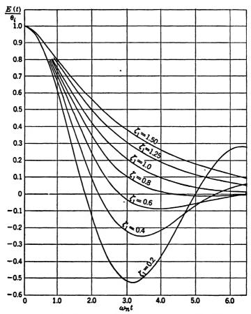
Fig. 9-6.—Dimensionless transient error curves of a servomechanism with a Type 1 controller when subjected to a suddenly applied input angle  $\theta$ . (Courtesy of G. S. Brown, Transient Behavior and Design of Servomechanisms, Massachusetts Institute of Technology, 1941 and 1943.)
