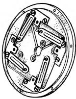
Fig. 5·18.—Sinusoidal potentiometer, type RL 14. The performance is indicated by the following data: angular resolution  $\pm \frac{1}{2}$ °; life  $5 \times 10^4$  revolutions at speeds up to 120 rpm; weight 1 lb 6 oz; diameter  $4\frac{3}{4}$  in.; length  $4\frac{1}{4}$  in.; winding resistance 32,000 ohms; applied voltage 300 volts or less; 305 turns per inch of 0.0025 = in. diameter nichrome wire; Formex insulation; brush force 1 oz; and resolution 0.3 per cent of peak voltage.
