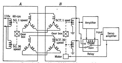
Fig. 12-7.—Servo with 1- and 36-speed data transmission.
