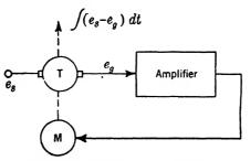
Fig. 4.29.—Velocity servo integrator.
