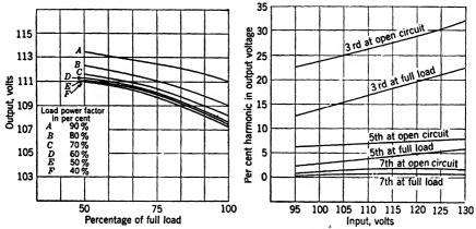
Fig. 16·16.—Output voltage vs. percentage of full load at various load power factors for a standard 500-volt-ampere voltage stabilizer. Input, 115 volts; nominal output, 115 volts.
