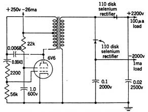
Fig. 16-52.—Schematic of 2 ky a-f high-voltage supply.
