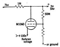
Fig. 16.54.—Degenerative shunt high-voltage regulator.
