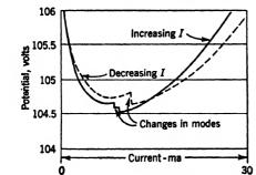
Fig. 15-4.—Volt-ampere characteristics of VR-105 for increasing and decreasing current.
