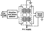
Fig. 12-62.—Use of saturable transformer in servo system.
