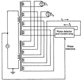
Fig. 3-12.—Saturable core current discriminator circuit.
