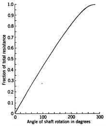
Fig. 5.1.—Function wound on a nonlinear potentiometer.
