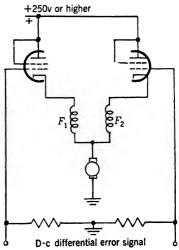
Fig. 12-42.—Circuit for vacuumtube control of split-series motor from d-c power supply.
