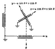
Fig. 6.23.—Rotation of coordinates by a resolver.
