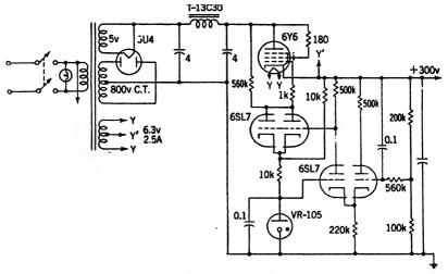
Fig. 16.28.—Balanced comparison circuit.
