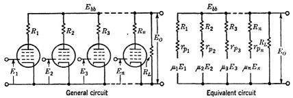
Fig. 3.9.—Common plate-load addition.
