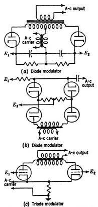
Fig. 15-21.—Vacuum-tube modulators.
