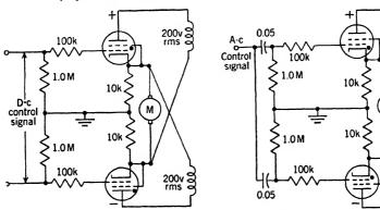
Fig. 12-27.—Circuit for thyratron bidirectional control of motor armature from d-c error signal.
