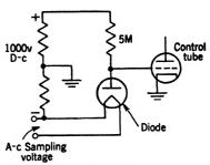
Fig. 15.16.—Bridge circuit for diode emission reference element.
