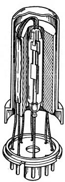
Fig. 12.50.—Western Electric D-168479 mercury contact relay.
