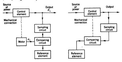
(a) Motor actuated control element
