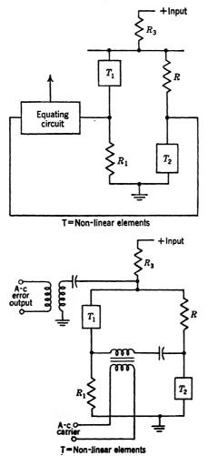
Fig. 15-18.—Sampling circuits with nonlinear elements.
