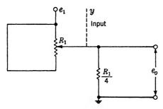
Fig. 5-10.—Circuit for approximating secant.
