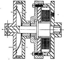
Fig. 12-22.—Fixed-coil friction-type magnetic clutch.
