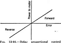
Fig. 12.44.—Relay proportional control characteristic.
