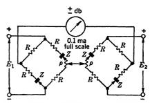
Fig. 5.36.—Combination of logarithmic bridges for division.
