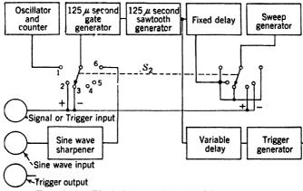
Fig. 18-10.—Block diagram of the Model 5 synchroscope.
