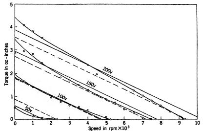
Fig. 13-1.—Speed-torque curves at various d-c control voltages for Elinco Midget type MS-1 motor. Broken straight lines show assumed linear characteristics.
