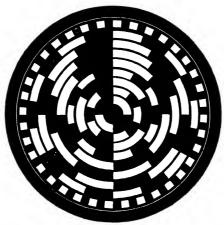
Fig. 13-3.—Stroboscope disk for speed measurements.
