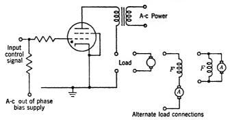
Fig. 12-29. -A basic thyratron motor-control circuit.
