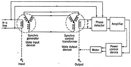
Fig. 8.1.—Simple remote follow-up servomechanism.
