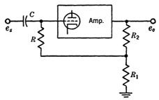
Fig. 4-4.—Increase of output by attenuation of feedback.
