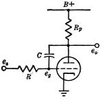
Fig. 4.23.—One-tube integrator.
