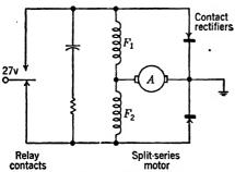
Fig. 12.54.— Relay contact protection with small rectifiers.
