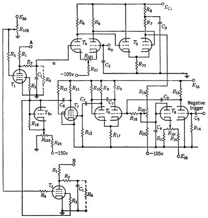
Fig. 3-14.—Pulsed attenuator computer schematic.
