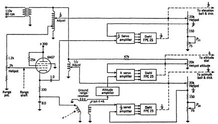
Fig. 7-22.--Ground-range resolver and servo channels.
