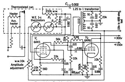
Fig. 16.24.—Precision 350-cps oscillator.
