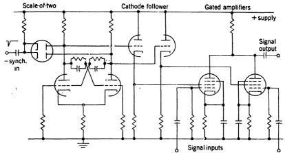
Fig. 17-13.—Electronic switch for video signals.
