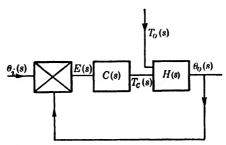
Fig. 9-8.—Block diagram of a serve system involving an output disturbance  $T_0(s)$ . the procedure previously discussed (page 239) is applicable regardless of the nature of the input function.
