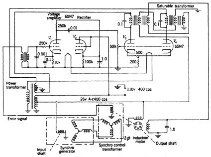
Fig. 12-63.—A 400-cps servo using Bendix saturable transformer.
