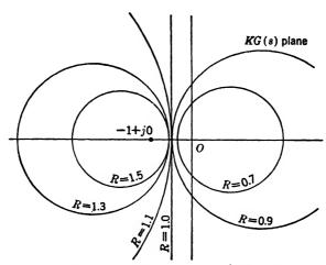
Fig. 10-19.—Transfer locus corresponding to constant  $|\theta_0(j\omega)/\theta_i(j\omega)|$  ratios. (Based on Harris, "The Analysis and Design of Servomechanisms," NDRC Report, 1942, Fig. 25.)
