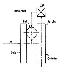
Fig. 4.18.— Ball-and-disk integrator as a differentiator.
