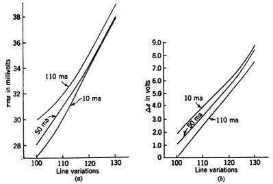
Fig. 16-39.—Characteristics of Oregon Electronics supply. (a) Output ripple; (b) change in output voltage.
