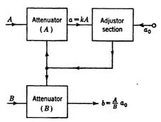
Fig. 3-13.—Pulsed attenuator computer block diagram.
