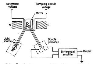
Fig. 15-26.—Use of galvanometer and photocells in comparison circuit.
