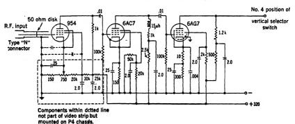
Fig. 18-5 .- P4E amplifier circuit.
