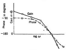
Fig. 10·17.—Decibel vs. log frequency diagram of a system just as the boundary line between stability and instability. Gain and phase margins are zero.
