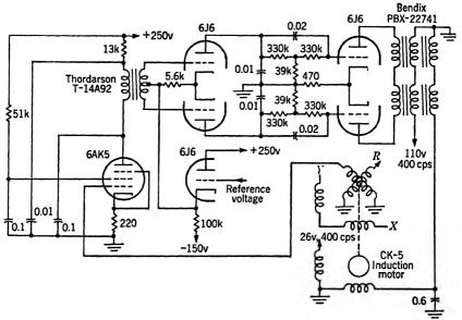
Fig. 14.7.—Detailed schematic of resolver servo.
