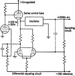
Fig. 16-53.—Oscillator high-voltage supply with d-c regulator.
