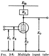
Fig. 3.8. Multiple input tu adding circuit.
