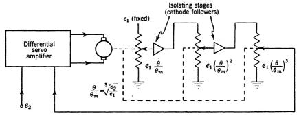
Fig. 5-31.—Device for producing cube root.
