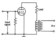
Fig. 12-24.—Simple thyratron control circuit.
