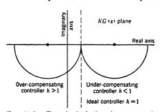
Fig. 11.8.—Transfer loci of various types of integral controllers.
