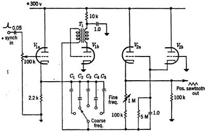
Fig. 17-2.—Free-running blocking-oscillator sweep generator.
