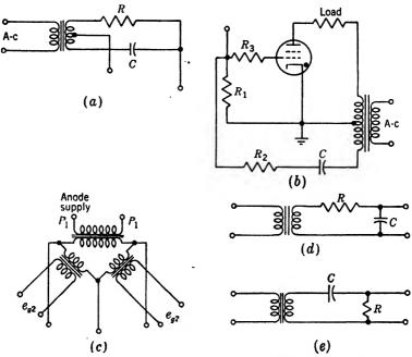
Fig. 12.26. —Practical circuits for securing phase-shifted a-c bias.
