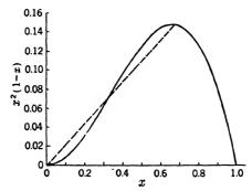
Fig. 5-8.—Potentiometer loading curve for  $\alpha \gg 1$ .
