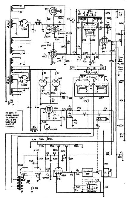
Fig. 16-31.—Precision d-c voltage supply.
