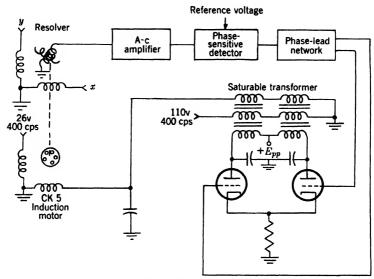
Fig. 14.5.—Detailed schematic of resolver servo.
