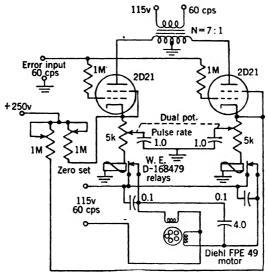
Fig. 12.65.—Simple thyratron and relay control for a-c motors.
