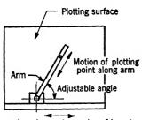
Motion of arm along edge of board Fig. 6.29.—Plotting board with two mechanical motions at adjustable angle.
