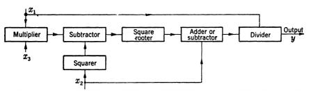
Fig. 6.2.—Block diagrams for solution of quadratic equation. (a) Solution of the implicit function  $x_1y^2 + x_2y + x_3 = 0$  by feedback; (b) solution of  $x_1y^2 + x_2y + x_3 = 0$  using the explicit function  $y = \frac{-x_2 \pm \sqrt{x_2^2 - 4x_1x_3}}{2x_1}$ .
