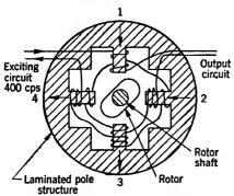
Fig. 12.3.—Schematic diagram of Microsyn.
