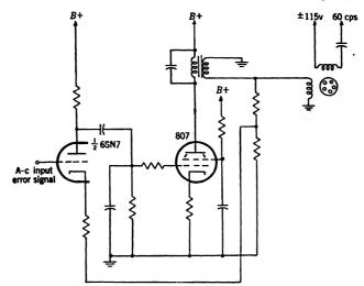
Fig. 12.58,—Single-ended motor power-control stage.
