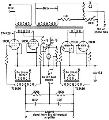
Fig. 12:32.—Push-pull bidirectional thyratron control circuit for Elinco MS-2 or FB split-series motor.
