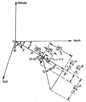
Fig. 7:11.—Ground plane geometry including wind and site motion.
