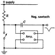
Fig. 17-4.—Sweep generator using negative feedback for linearization.
