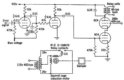
Fig. 12-67.—Relay servo for Bendix CK-1 motor. This somewhat unusual servo is operated at high gain, hunting steadily at about  $\frac{1}{10}$ ° amplitude.
