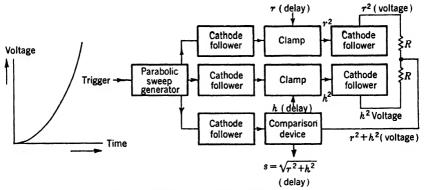
Fig. 6.6.—Hypothetical parabolic-sweep triangle solver.
