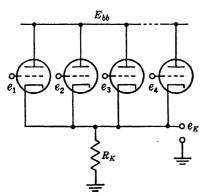
Fig. 3-10.—Common cathode-load addition.
