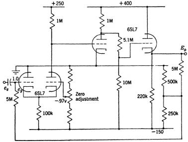
Fig. 4.6.—Example of feedback amplifier type of RC-differentiator.
