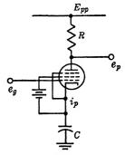
Fig. 4.8.—C at hode follower differentiator using pentode with separate screen supply.
