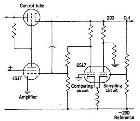
Fig. 16-32.—Alternate circuit for +200-volt regulator.
