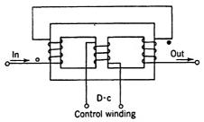
Fig. 15.29.—Saturable reactor with d-e control.
