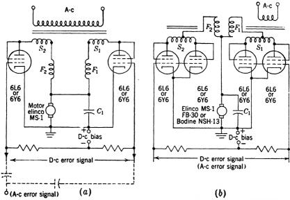
Fig. 12·35.—Control of split-series d-c motor by vacuum tubes. (a) Half-wave drive; (b) full-wave drive. Either d-c or a-c error signals may be used.
