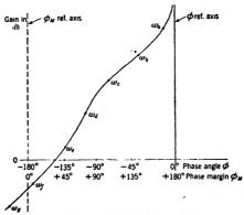
Fig. 10-8.—Phase-margin diagram.
