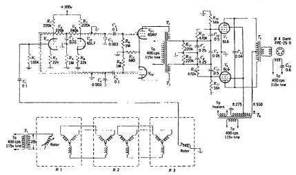
Fig. 14.4.—Schematic of PP1 follow-up servo.
