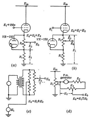
Fig. 3.4.—Addition or subtraction with series sources.
