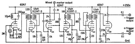
Fig. 18-52.—Crystal-controlled marker generator circuit.
