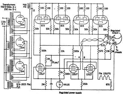
Fig. 16.47.—Regulated power supply.
