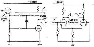
Fig. 17.6 .- Negative-feedback inverter.
