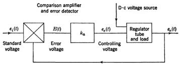
Fig. 10-14. - Block diagram of voltage regulator.
