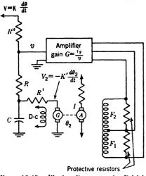
Fig. 12·40.—Block diagram of British Velodyne circuit.
