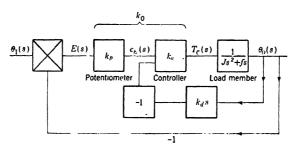
Fig. 11.5.—Proportional servo system with tachometer feedback.
