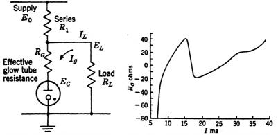
Fig. 16.3.—Simple glow tube regulator.
