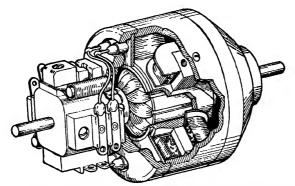
Fig. 12·17.—Lightweight field-controlled d-e motor, Holtzer Cabot RBD 0808.
