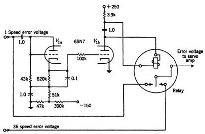
Fig. 12·8.—Amplifier and relay for synchronizing multispeed servo system.
