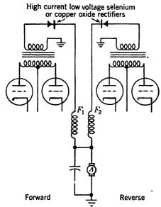
Fig. 12.41.—Transformer and contact rectifier control circuit for split-series d-c motor.
