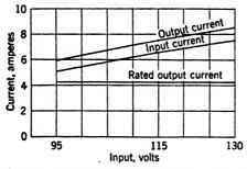
Fig. 16-18.—Input and output current under short-circuit conditions as a function of input voltage for a standard 500-volt-ampere voltage stabilizer.
