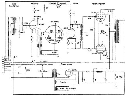
Fig. 7.21.—Servo schematic.
