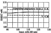
Fig. 16·13.—Output voltage vs. input voltage for 500-volt-ampere unit at rated unity power factor load. Data subject to 1 per cent manufacturers' tolerance.
