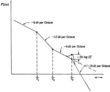
Fig. 10-7.—Asymptotic gain curve for transfer function:
