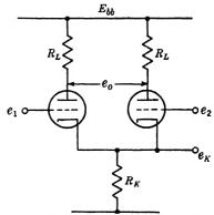
Fig. 3-11.—Differential amplifier for adding and subtracting.
