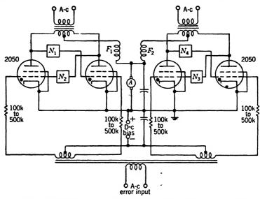
Fig. 12-33.—Bidirectional push-pull thyratron motor-control circuit with a-c error signal for split-series motor. Out-of-phase bias is supplied by networks  $N_1$ ,  $N_2$ ,  $N_3$ , and  $N_4$ .
