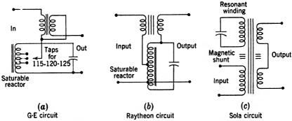
Fig. 16·12.—Commercial constant-voltage transformers.
