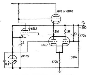
Fig. 16.27.—Balanced comparison circuit.
