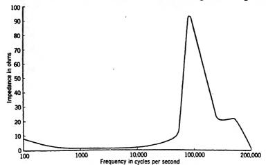
Fig. 16.46.—Output impedance vs. frequency for regulator C.
