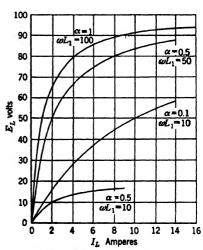
(b) Characteristics for saturable reactor,  $E_L = \frac{\omega L_1 I_L}{1 + \alpha I_r}, \quad L_0 = \frac{L_1}{1 + \alpha I_r}$
