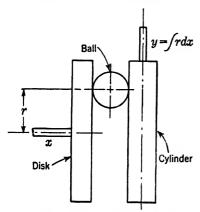
Fig. 4.34.—Ball-and-disk integrator.
