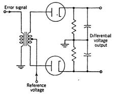
Fig. 12-14.—Phase detector using addition of voltages.
