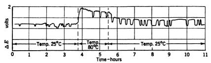
Fig. 15.5.—Time, voltage, and temperature characteristics of a glow tube. Tube switched off for 20 sec every 4 min.
