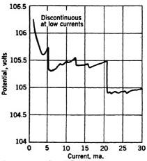
Fig. 15-3.—OC-3 (VR-105) glow tube voltampere characteristics.
