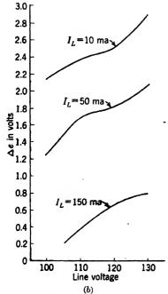
Fig. 16.40.—Characteristics of laboratory power supply. (a) Output ripple; (b) output voltage.
