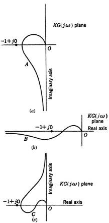
Fig. 10-15. Transfer locus diagrams representing systems with zero steady-state errors.
