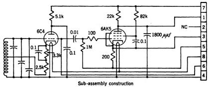
Fig. 19-21.—Circuit of 20-kc oscillator subassembly.
