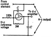
Fig. 15.27.—Diode detector equating circuit.
