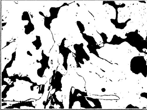
0.20 Per Cent Carbon Steel—white, ferrite—black, pearlite—100x.
