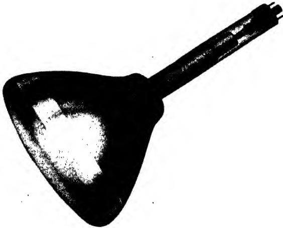
FIG. 3.2B. MAZDA CRM 121 (TWELVE-INCH) PICTURE TUBE (Courtesy of Edison Swan Electric Co., Ltd.)
