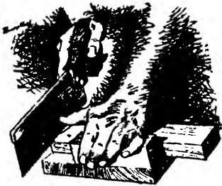
Fig. 6. Starting the cut with a tenon saw. The work is held on a bench hook. Note specially how the thumb bears against the blade of the saw.
