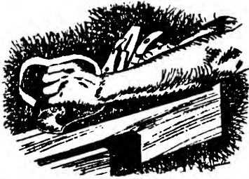
Fig. 14. Shooting or planing the edge of a board. Sometimes the fingers curl beneath the sole of the plane, acting as a fence.
