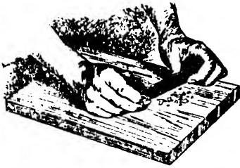
Fig. 30. Method of using the hand scraper on hardwood panel.
