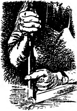
Fig. 27. Vertical paring with chisel. In all chiselling work both hands must be kept behind the cutting edge.
