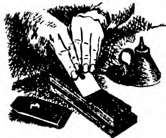
Fig. 17. Sharpening a plane iron on oilstone. Note the manner of holding the blade to maintain an even pressure.
