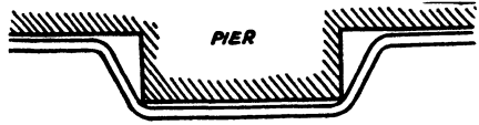
Fig. 17.—A BETTER METHOD, USING A DOUBLE OFFSET WHICH AVOIDS FITTINGS AND REDUCES FRICTION
