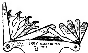
This Terry tool combines the essential equipment for distributor or magneto maintenance.
