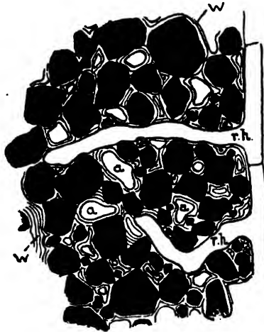
FIG. 17.—Diagram of soil with root-hairs ( r.h. ) to show the distribution of air ( a ) and water ( w ) (much enlarged). Soil-particles in black.
