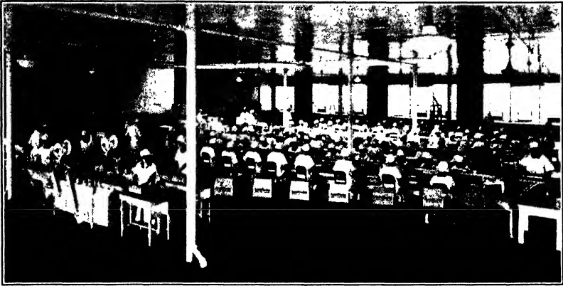
FIG. 87. Printing butter. Spacious, sanitary butter-printing room in the Land O' Lakes plant, Minneapolis, Minn. Note the automatic printing and wrapping machines at the left. The girls seated at the long tables wrap and carton pound prints of butter coming from hydraulic presses.
