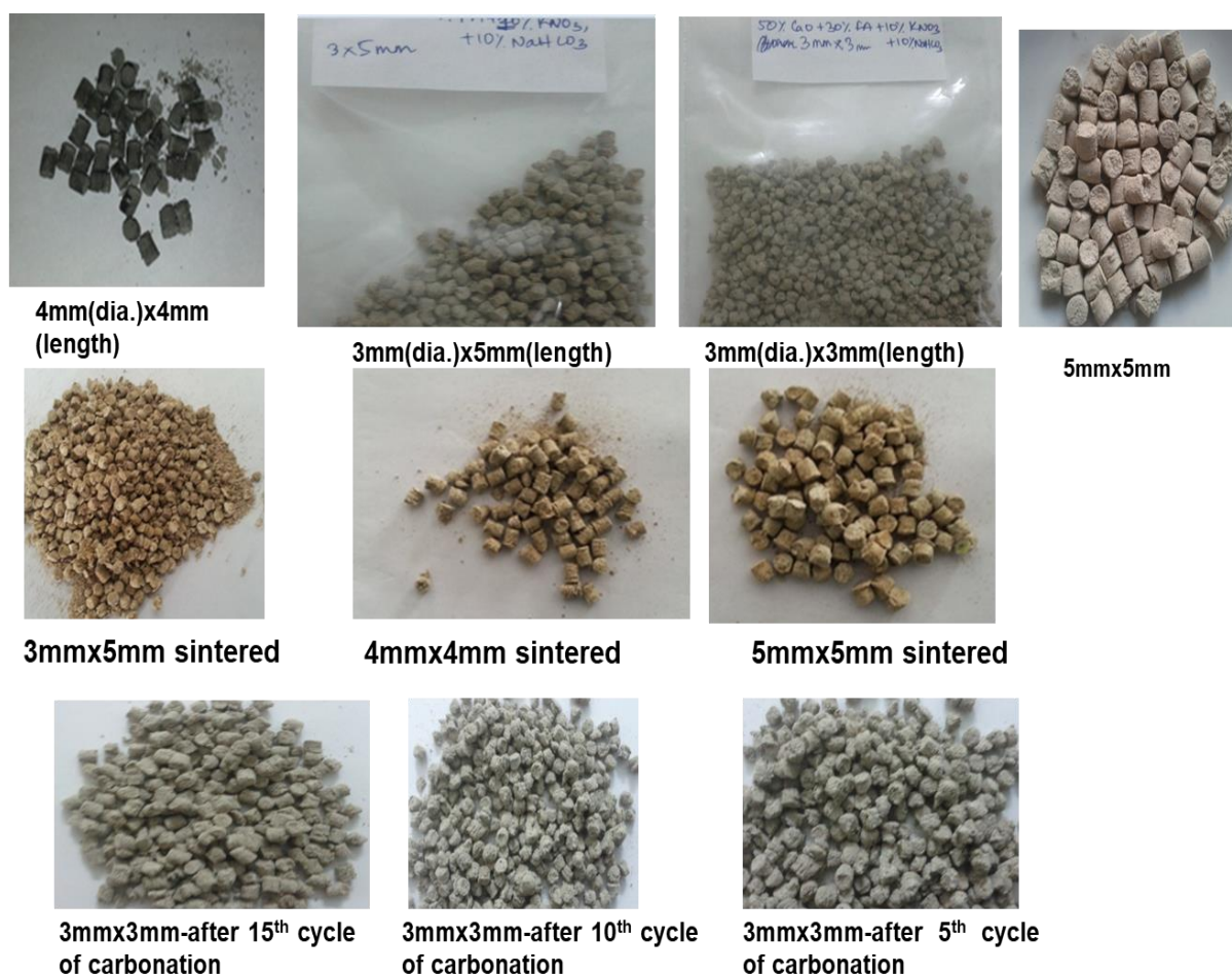
Figure 2.10 Monolithic granule sizes of sorbents synthesized
