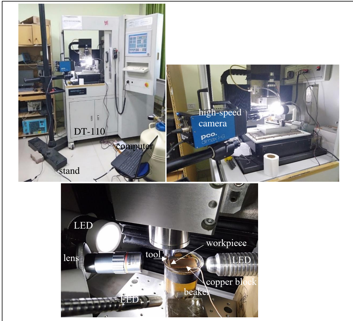
Figure 6.10 Experimental setup on DT-110 with pco. dimax HS4 high speed camera
