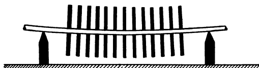
(a) Long shafts bend between points of support as at bearings, because of their own weight (grossly exaggerated)
