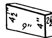
NO. 1 KEY 9 \times (4\frac{1}{2} - 4) \times 2\frac{1}{2} in. 113 brick to the circle 12 ft. I.D.; 13\frac{1}{2} ft. O.D.
