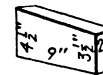
NO. 2 KEY 9 \times (4\frac{1}{2} - 3\frac{1}{2}) \times 2\frac{1}{2} in. 57 brick to the circle 5\frac{1}{4} ft. I.D.; 6\frac{3}{4} ft. O.D.
