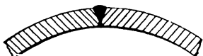
FIG. 191.—Boiler drum showing butt double-welded joint reinforced at center as required by the boiler code.
