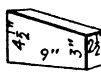
NO. 3 KEY 9 \times (4\frac{1}{2} - 3) \times 2\frac{1}{2} in. 38 brick to the circle 3 ft. I.D.; 4\frac{1}{2} ft. O.D.
