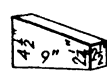
NO. 4 KEY 9 \times (4\frac{1}{2} - 2\frac{1}{4}) \times 2\frac{1}{2} in. 25 brick to the circle 1\frac{1}{2} ft. I.D.; 3 ft. O.D.
