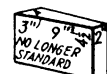
NO. 3 WEDGE 9 \times 4\frac{1}{2} \times (3 - 2) in. 57 brick to the circle 3 ft. I.D.; 4\frac{1}{2} ft. O.D.
