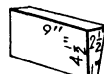
NO. 3 ARCH 9 \times 4\frac{1}{2} \times (2\frac{1}{2} - 1) in. 19 brick to the circle 6 in. I.D.; 1\frac{1}{4} ft. O.D.
