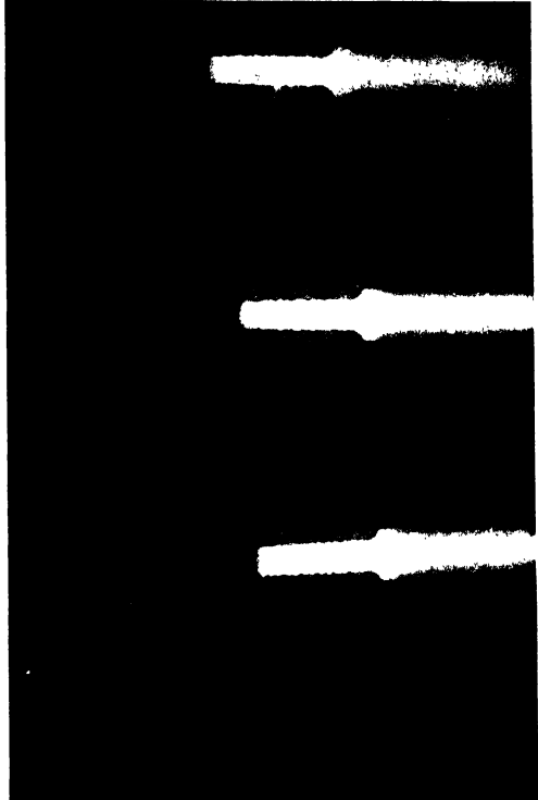
FIG. 28. MAGNESIUM-RICH ALLOY CASTING CONTAINING A STEEL INSERTION
