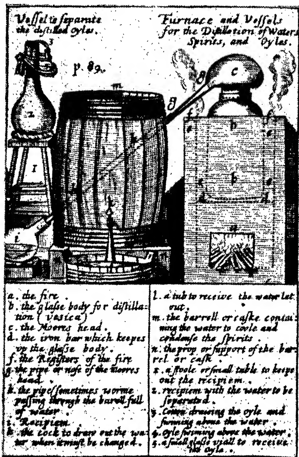
28. Steam-distilling Essential Oils of Plants. After N. le Febure, 1664
