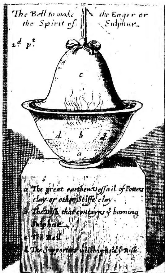
26. The Preparation of Spirit of Sulphur per campanam . After N. le Febure, 1664
