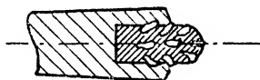
FIG. 162.—Diamond chips embedded in a tungsten or tungsten carbide matrix; tool used for truing purposes
