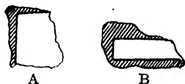
FIG. 148.—A and B. Cutting industrial diamonds according to the shape of the rough stone is not a satisfactory method
