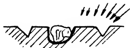
FIG. 164.—Caulking (peening) of a rough diamond for setting in a rock-drill crown
