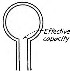
FIG. 59.—Sketch of magnetic dipole antenna.
