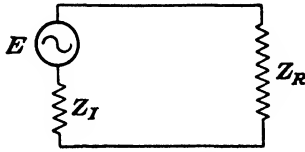
FIG. 16.—A generator connected to a load.
