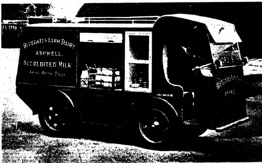
Fig. 34. —AN 8/10-CWT. MURPHY ELECTRIC With body designed for the delivery of dairy produce.
