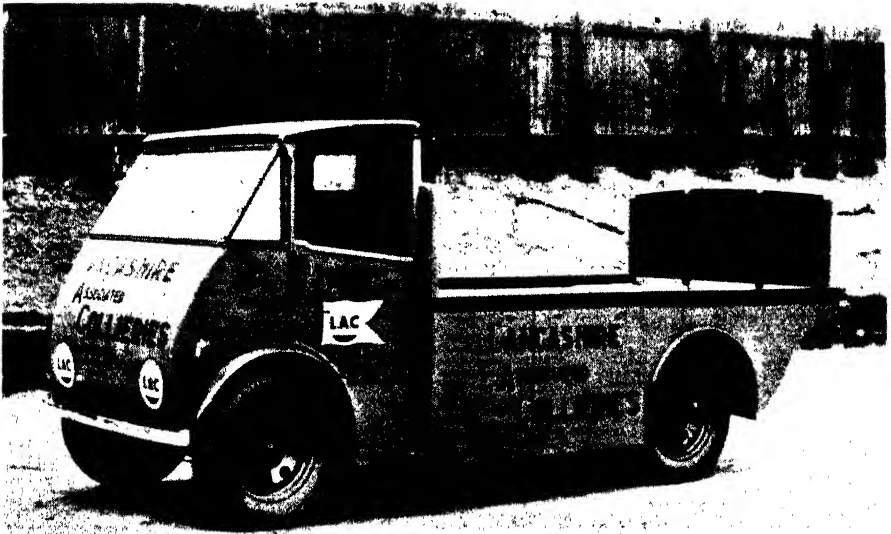
Fig. 30. —A MIDLAND ELECTRIC MODEL B20, 18/22-CWT. PAYLOAD With platform-type body for coal delivery.
