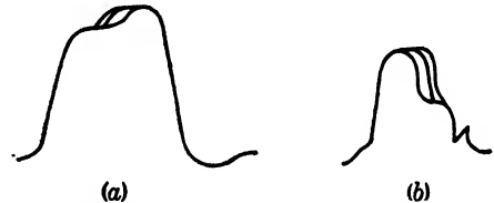
FIG. 8.10.—The pulses of (a) voltage and (b) current that are associated with a mode shift.
