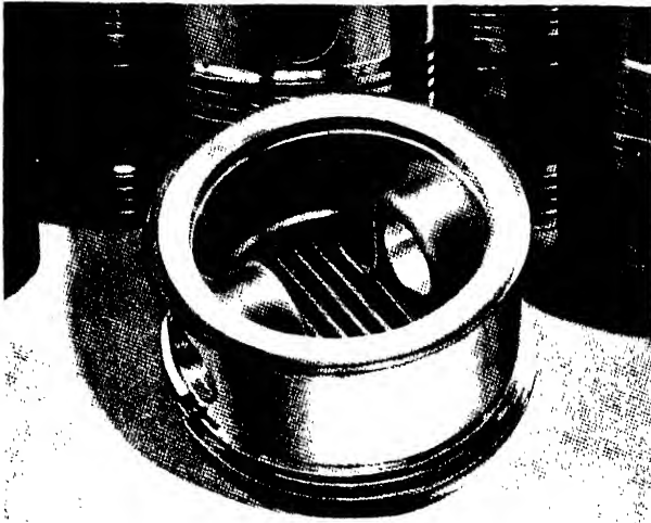
FIG. 197. Piston of Pratt and Whitney Twin "Wasp" engine.
