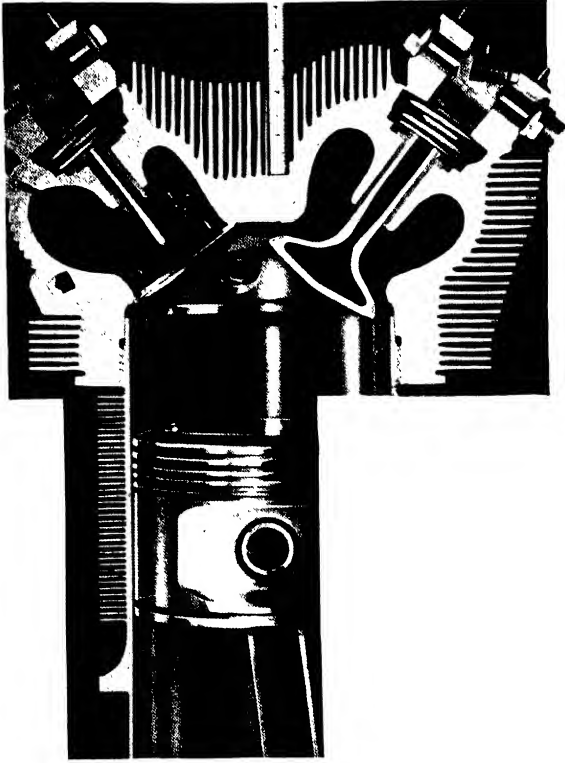
FIG. 101. Sectional view of Wright "Cyclone" G-200 cylinder, showing cooling fins and valves.
