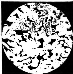
Fig. 42. 0.2% carbon steel forging normalised, showing pearlite and ferrite. \times 100
