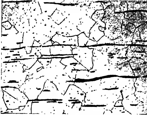
Fig. 40. Wrought iron, showing grains of ferrite and slag inclusions. \times 100
