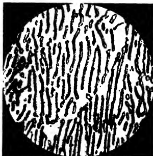
Fig. 44. 0.8% carbon tool steel, annealed. \times 2500
