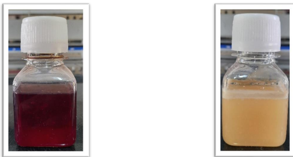
a) The initial state of culture medium b) Final state of culture medium (if bacteria is present)
